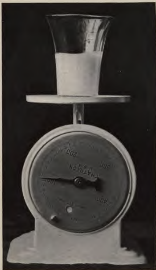
Fig. 1.—Chatillon gram scales with movable disk. A counter-weighted balance convenient for weighing food. An empty glass was placed on the scale pan. The dial was turned by means of the knob, so that its 0 point coincided with the pointer. Milk was then poured into the glass until the pointer stood at 105, the amount of milk desired for a certain diet.
